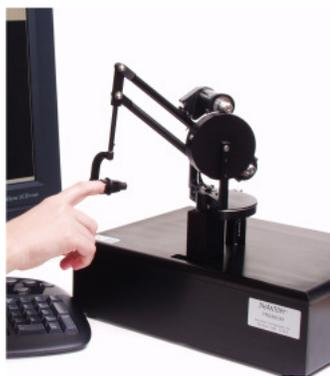
Figure 5.13: SensAble Phantom haptic robotic arm
