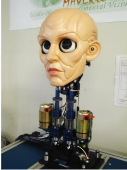
Figure 3.4: Robotic oculomotor vision head by Sarcos (Cambridge, MA).
