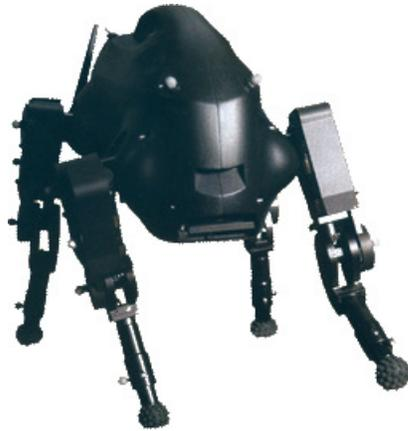
Figure 4.4: LittleDog quadruped robot by Boston Dynamics (Cambridge, MA).
