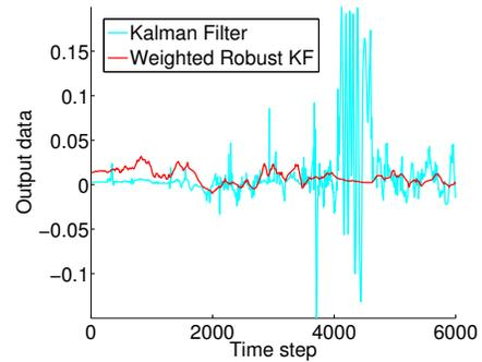
(b) Predicted data for the Kalman filter and weighted robust Kalman filter. Note the change of scale in axis from Figure 5(a).
