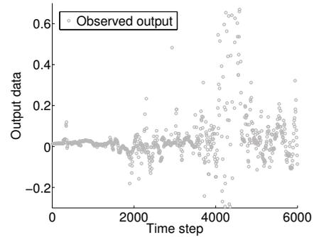
(a) Observed data,  $(q_{\text{IMU}} - q_{\text{MOCAP}})$ , from LittleDog robot: a slowly drifting noisy signal with outliers
